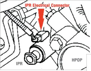
Disconnect the electrical connector from the injector pressure regulator.
