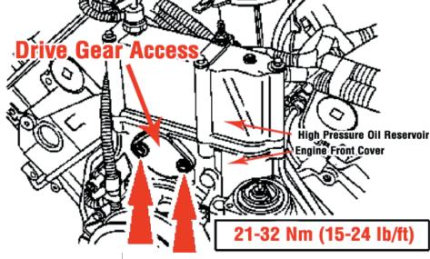
Remove the drive gear bolt (18mm) and washer from the drive gear.
