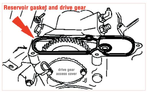
**CAUTION:** Make sure that the drive gear is fully seated on the high-pressure oil pump before installing the bolt and washer. Otherwise, the drive gear may not seat properly, causing binding or slippage resulting in a no oil flow condition. Do not assume the bolt will pull it tight and flush.
