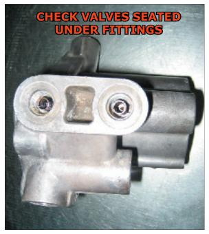
Remove the hoses from the high-pressure oil pump. Remove the two springs (check valves) found under the hose fittings.
