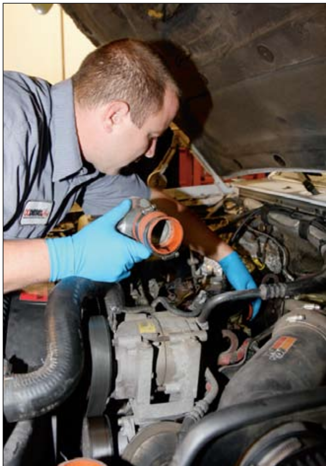
OC Diesel Shop's Matt Stranz performed the install and began by removing all of our intercooler plumbing and stuffed some paper towels into the intake manifold ports.
