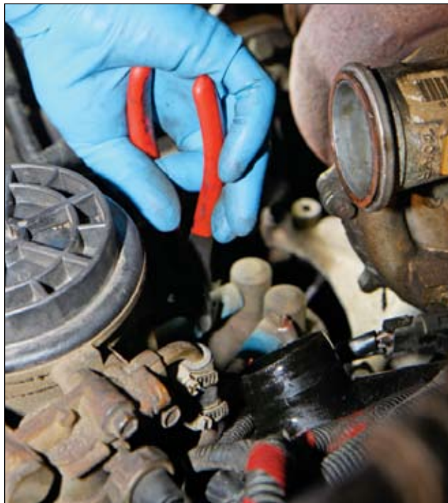
In order to remove the fuel bowl assembly and mechanical lift pump in the engine valley, the fuel lines running from the top of the lift pump to the fuel bowl were cut using a pair of pliers.
